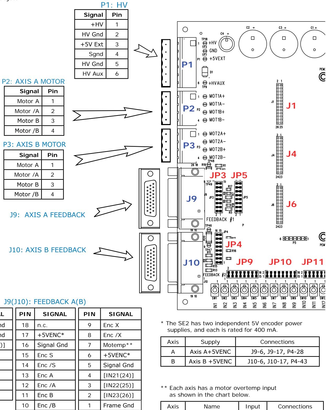
\* The SE2 has two independent 5V encoder power supplies, and each is rated for 400 mA.
